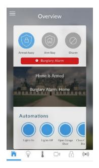
The menu bar is located along the bottom of the app. Touch the Zones icon (last icon with a dot and wireless signals) to view zone status.
