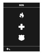
On this screen touch and hold the appropriate button for 2 seconds to activate Manual Fire Alarm, Manual Medical Alarm, or Manual Panic Alarm.
