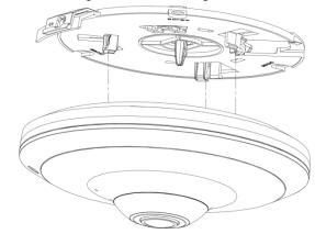
Step 6 Slide to lock the buckle on the mounting plate③. See Figure 3-4.
