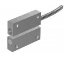
The MC 240-S45 set is intended for exposed environments where a more durable magnetic contact is needed, such as doors, gates, etc. The set consists of MC 240-C contact with a NC contact function installed in MC 200-4 Al housing and an extra strong magnet in MC 200-5 Al housing, which allows for a wide opening gap.
