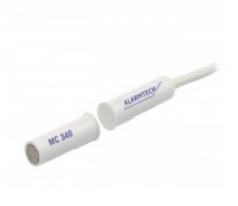
MC 340 is a universal magnetic contact with NC function that can be used in both alarm and access control systems for monitoring e.g. doors and windows against unauthorized opening. Both the contact and the magnet part are encased in a water proof (IP67) plastic housing, which enables easy installation into wood without additional accessories. With our extensive range of installation accessories it is easy to install the contact either recessed or as a surface mount on metal and other materials.
