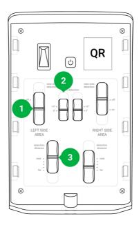
1. Near area detection switch for the left side of the detector
