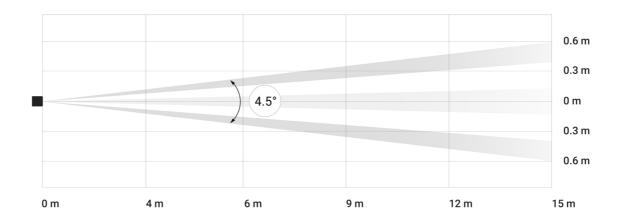
Horizontal viewing angle of the detector
