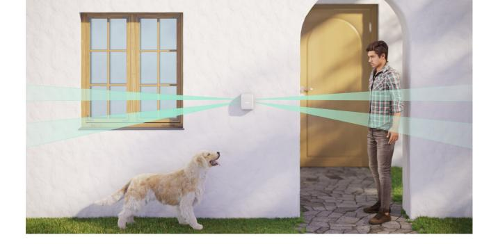
DualCurtain Outdoor is a bi-directional outdoor curtain motion detector. IR sensors of the detector identify intrusions by detecting moving objects with temperatures close to that of the human body.
