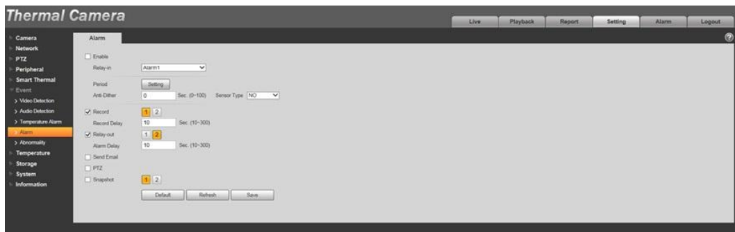
Figure 5-1 The alarm interface
