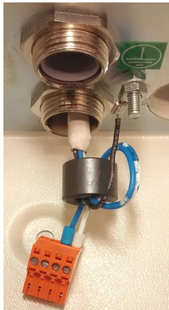
Figure 8: Looping relay connection wires around a suppression ferrite
