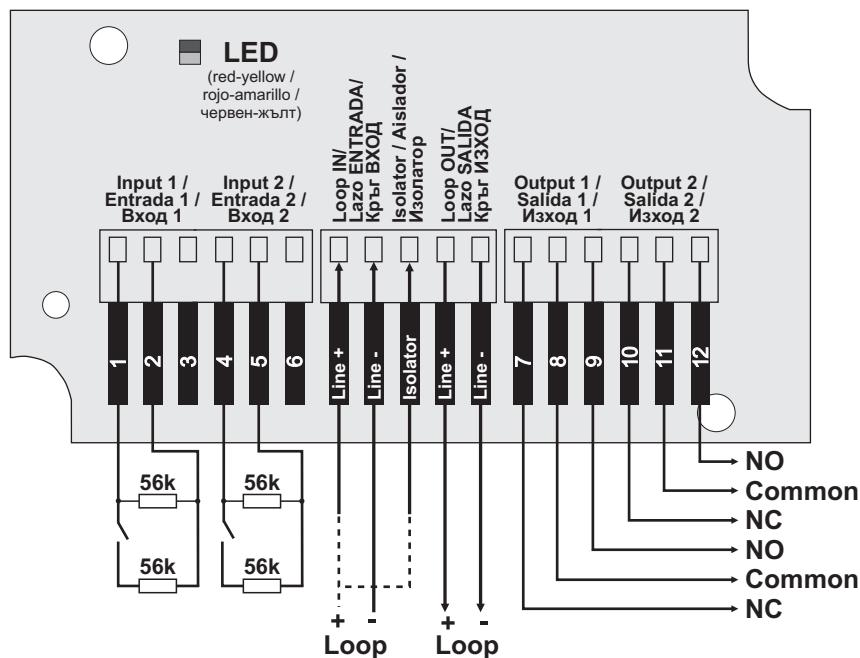
**ATTENTION:** When you use the integrated short circuit isolation module connect one of the "+Loop" loop lead to the "Isolator" terminal of the module.
