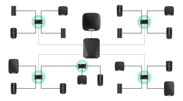
Connecting multiple LineSplit modules one after the other allows you to expand the Ajax system by splitting lines. One Fibra line splits into four, four into sixteen, and so on. The number of wired devices in the system is limited by the output current of the hub and its specifications. You can connect up to 100 devices to Hub Hybrid.
