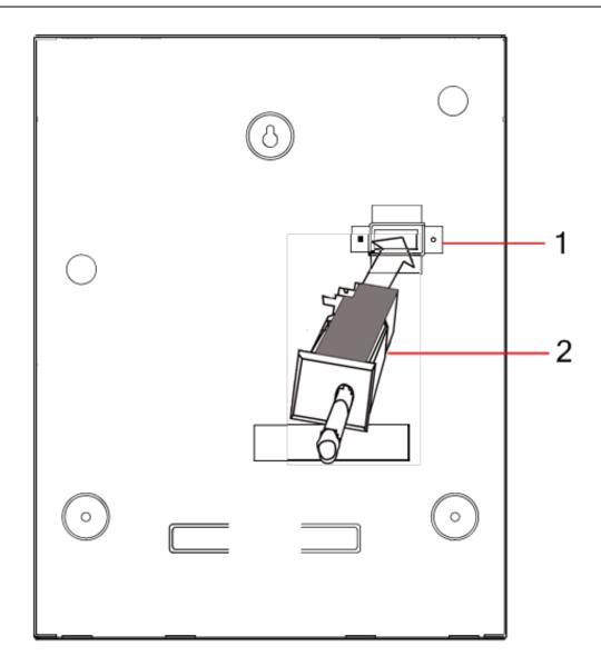
2. Fit the housing back onto the wall using the three fixings previously removed (see item 2 below). Visually check to ensure there is a flush finish between the wall plate and the housing metalwork.
