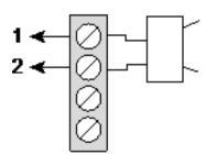
Internal sounder wiring (12V)
