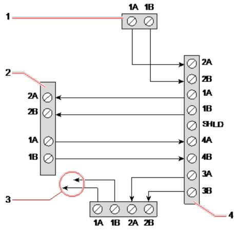
Wiring of a branch expander
