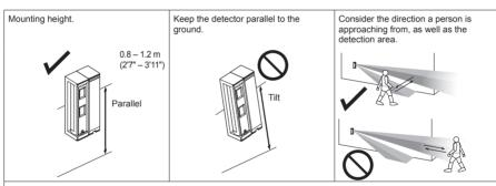
Install the detector in a place where it is free from false alarm factors. For example:
