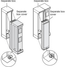
3 Connect the connector, and close the separate box.
