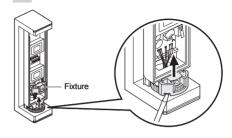
3 Hold the top of the bracket and remove the main unit.
