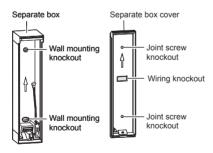
7 Pull the connectors through the wiring knockout.
