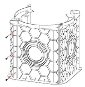
**3.** Enlarge the walls to allow to join the last section of the cablepit.
