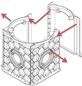
**4.** Insert and fix the screws in the other sides.
