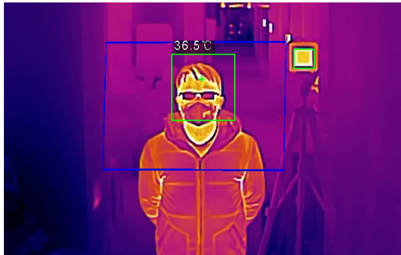
Figure 6-11 Adjusting TPC face detection box (2)
