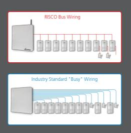
The RISCO Bus technology also enables system testing and diagnostic capabilities both locally and remotely through a choice of GPRS, IP and PSTN communication.
