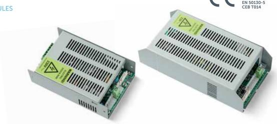
INIM offers two switching power supply/battery charger units: the 3A model and the 5A model. All models provide a thermal probe input. This device protects the batteries against overheating and consequent permanent damage by measuring the battery temperature and regulating the power supply output voltage accordingly.
