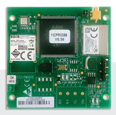
The WiFi Communication Module is a plug-in module enabling the connection of a ProSYS Plus, Agility or WiComm Pro Control Panel to an IP network via a WiFi router.
