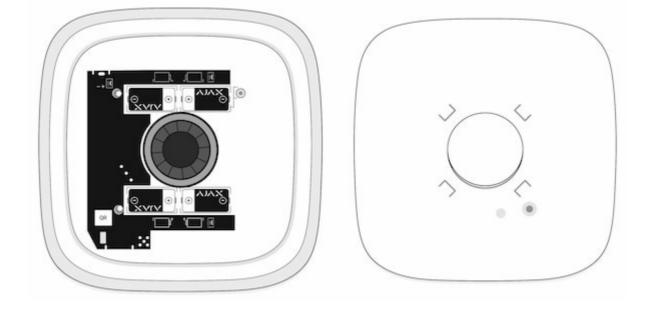
When installing the panel, do not remove the plastic frame and do not remove the LED strip from the seat!
