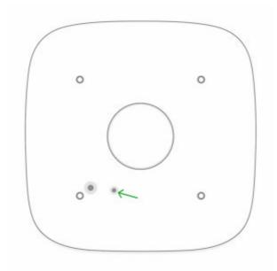
**11.** Fit the protective plastic panel in place (the Ajax logo on the connection side of the LED strip to the board) with little effort. The properly mounted plastic panel will protrude above the LED frame no more than 1.0 to 1.5 mm.
