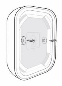
Do not use double-sided adhesive tape for either temporary or permanent mounting of the siren. The tape may break off under the weight of the siren. In addition, the tape dries up over time, which may cause the device to fall and the security system to trigger.
