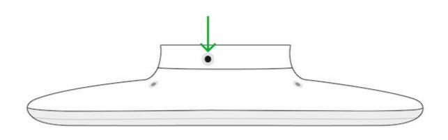
**3.** Remove the siren from the SmartBracket mounting panel, turning it counterclockwise if the siren is mounted on the mounting plate.
