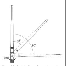
For achieving the best signal strength and coverage it is recommended the antenna to be mounted in straight up position!
