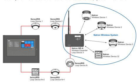
Up to 5 separate Natron WE-A modules can be connected in one iRIS8/iRIS4 system configuration. For optimum operation, plan to ensure at least 2m distance between two modules and the same minimal distance between each device and the module.
